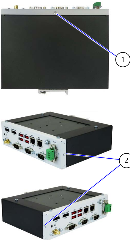
Figure 15: Front Panel Fastening Screws
