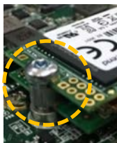
Figure 18: Fastening Screw M 2242/2280 and M.2 Key E 2230
