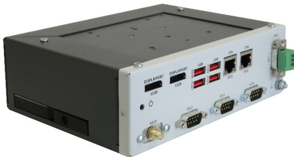
Figure 2: KBox A-150-WKL Drive Bay Variant with Wi-Fi and CAN Bus (options)
