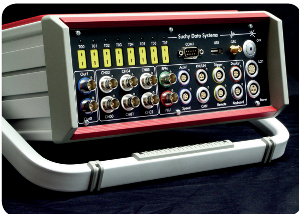
Figure 4: The Suchy testing system can process up to 600 dedicated measurement channels; the standard version provides 8 to 88 thermocouple inputs (yellow).
