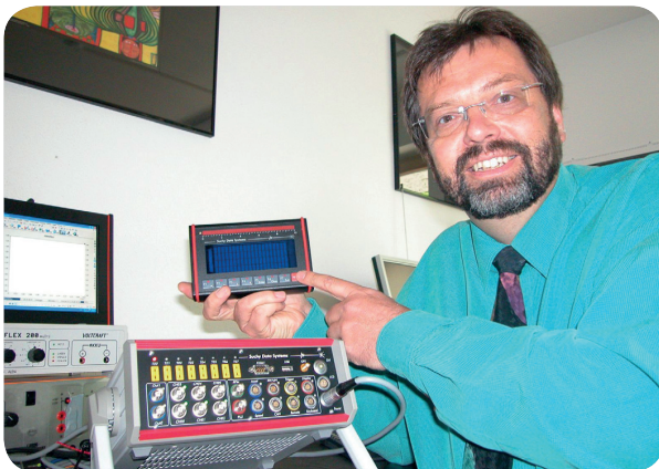
Figure 1: Manfred Suchy with testing system and driver display: The PC unit with the measurement electronics is located in a separate robust housing – all components are shock- and vibration-proof. The additional driver display consists of a large text display showing the most important measurement data and simultaneously serving as a menu navigator. In the background to the left: Sunlight-resistant monitor, which can be attached to the windshield via suction cups to give the driver a perfect view of it.
